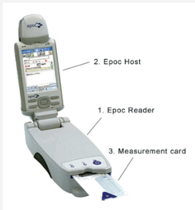
Picture 5. Portable blood gas and electrolyte analyzer (EPOC).
