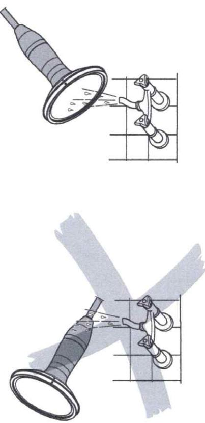
**⚠** Danger of electric shock! Make sure that no humidity enters the handpiece. Do not immerse the handpiece or plug.
