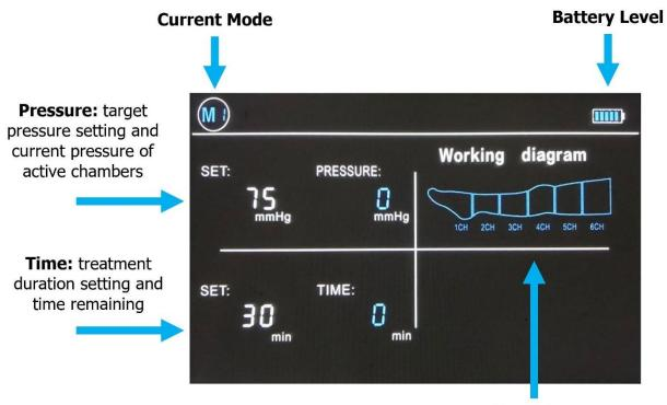
Working Diagram: active chambers are filled on the diagram (no active chambers in example)
