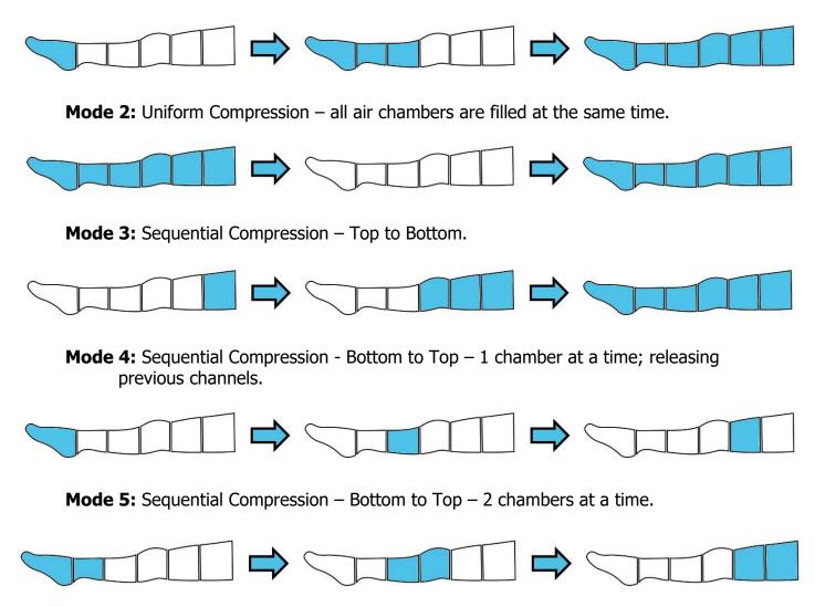
Note: The system will automatically default to Mode 1 / 75 mmHg / 30 min.
