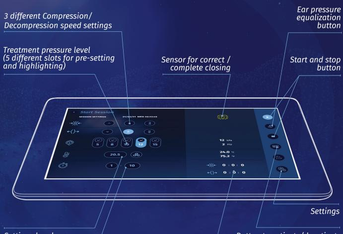
Setting chamber temperature Button to activate/deactivate the touch display inside the chamber
