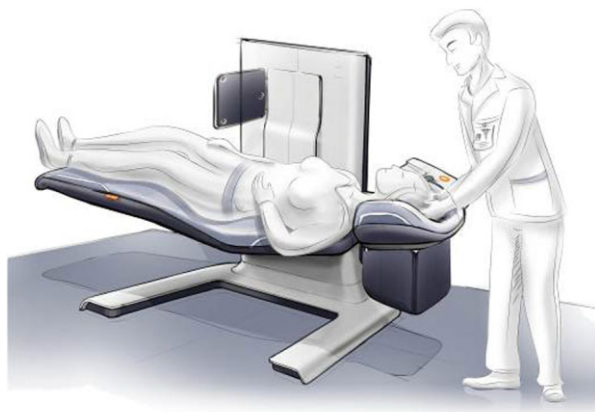
Figure 1 Sketch of the Occiflex device. Patient is lying on treatment table (left) and therapist standing beside.
